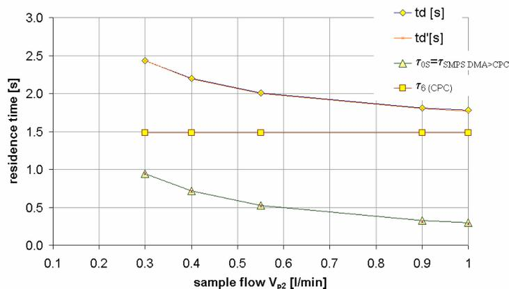
Figure 29 Residence time for the CPC3010 and the standard SMPS tubing as a function of the sample flow  $V_{P1}$  (description see text).
