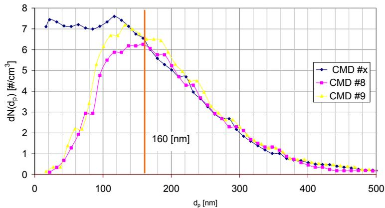
Figure 35 CMD measurement one day after the soot measurements of experiment #65 with the same aerosol enclosed (experiment #67); the numbers #x refer to the usual different first measurement and #8-9 to the single measurement run of the monodisperse measurements (see Table 16); Dilution with ambient air had occurred .
