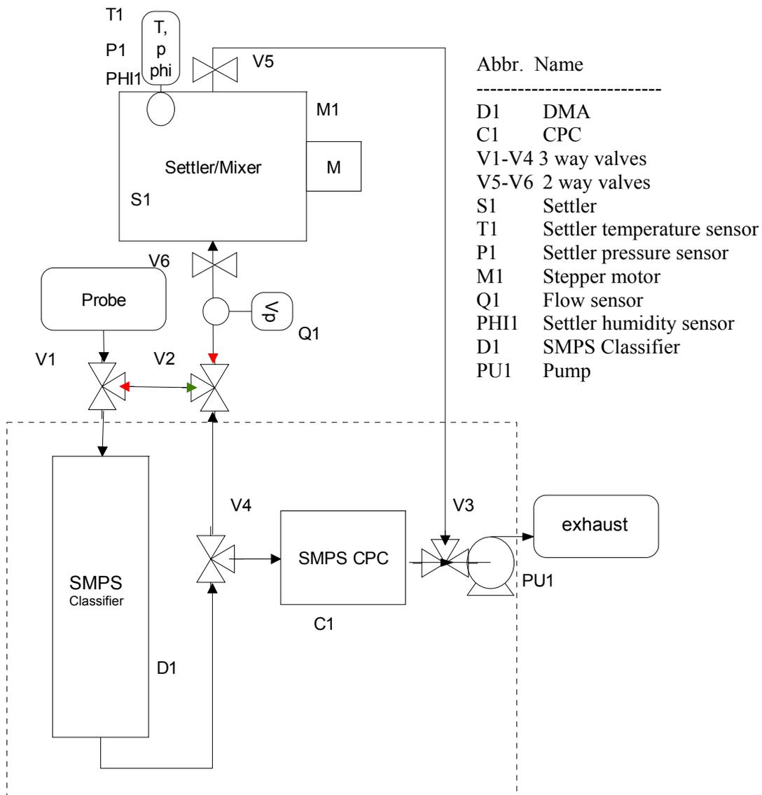
Figure 7 Basic Setup of the CMD
