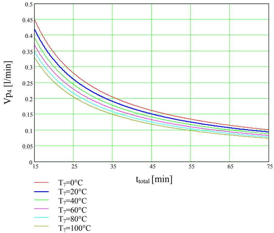
Figure 16 Volume flow  $V_{p4}$  at  $T_4=20^\circ\text{C}$  as a function of different settler temperatures  $T_7$  and the total measurement time  $t_{total}$ . The ambient temperature  $T_2$  is also  $20^\circ\text{C}$ .
