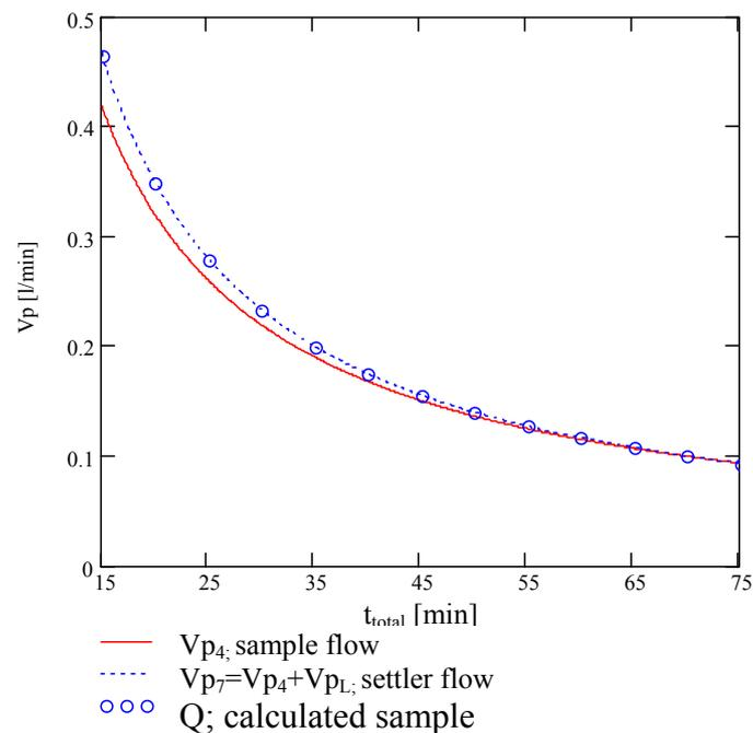
*Figure 12 Settler flow rates as a function of the total time for pressing out the complete settler volume;  $V_{p4}$  is according to the measurement in Figure 11; The measured flow together with the calculated leakage flow  $V_{p7}$  (see text) is shown with the blue dotted line and shows a good accordance with the volume flow  $Q$  calculated from the settler geometry according to equation (0-4).*
