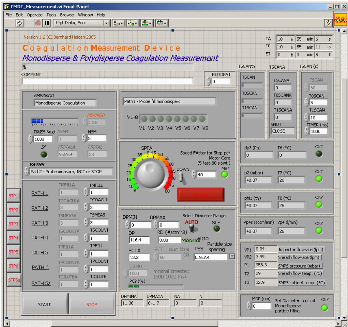
Figure 25 Application window of the CMD-Program: "CMDC\_Measurement.vi"; this is the central window controlling all measurements
