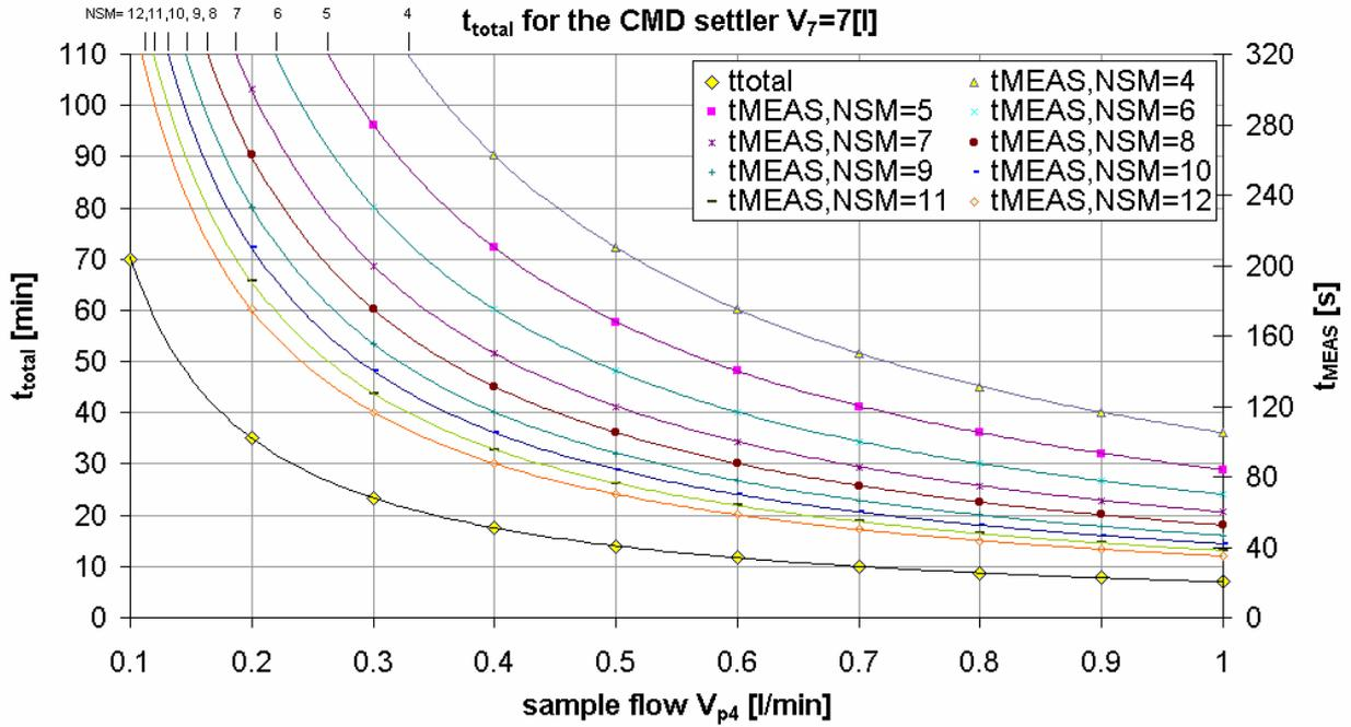
Figure 27 Total measurement time possible when emptying the settler as a function of the sample flow  $V_{p4}$  and the number of the measurements (NSM) on the right y-axis; The total measurement time as a function of  $V_{p4}$  can be read on the left y-axis (calculation see equation (0-20)).
