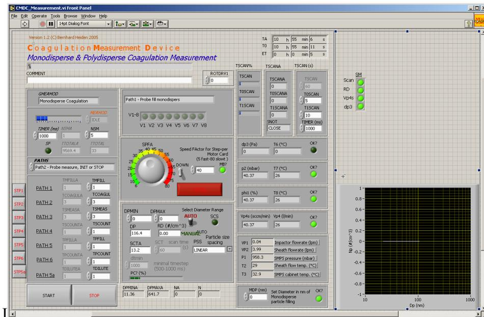
Figure 50 Detailed front panel of the main measurement program: *CMDC\_Menu.vi*
