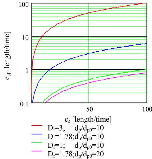
*Figure 1* Corrected settling factor  $c_{sf}$  for fractal particles as a function of the settling velocity  $c_s$  for spherical particles. Decreasing fractal dimension  $D_f$  and decreasing particle size  $d_p$  leads to a decreasing settling velocity. The value  $D_f=1.78$  is the value for Brownian coagulation in the three dimensional space often applied for soot particles (Jullien and Botet 1987) p.88.
