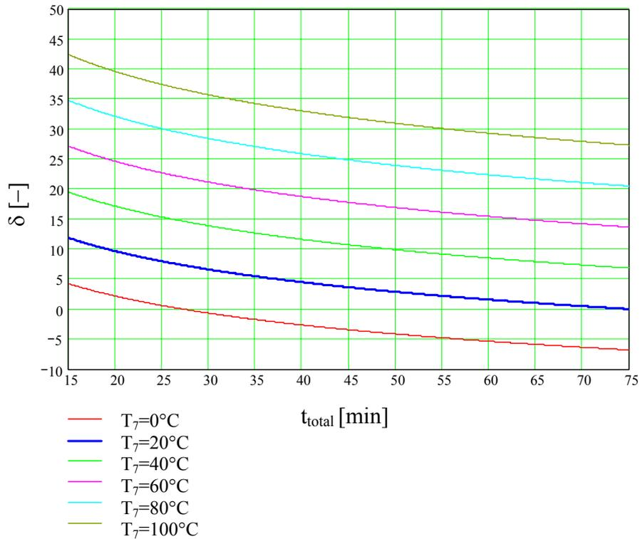
Figure 17  $\delta$  in % at  $T_4=20^\circ\text{C}$  as a function of different settler temperatures  $T_7$  and the total measurement time  $t_{total}$ . The ambient temperature  $T_2$  is also  $20^\circ\text{C}$ .
