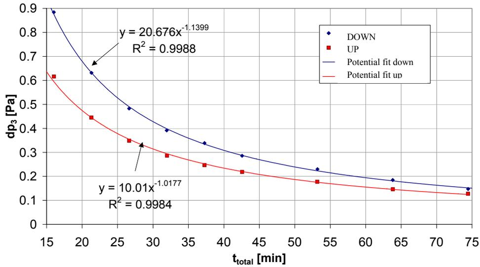
Figure 15 Pressure difference measurements for the sensor ASP 1400 for different times of emptying and filling the settler.
