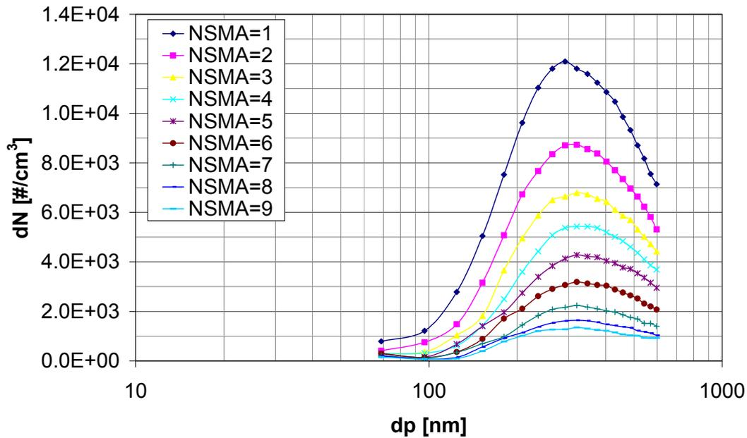
Figure 38 Sized distributions measured with the CMD for the incense measurements for nine sequential runs  $NSMA=1..9$  in the CMD operation “Polydisperse Coagulation”.  $dN$  is the particle size measured with the CPC plus the correction for the dilution and  $d_p$  is the mobility particle diameter in nm.
