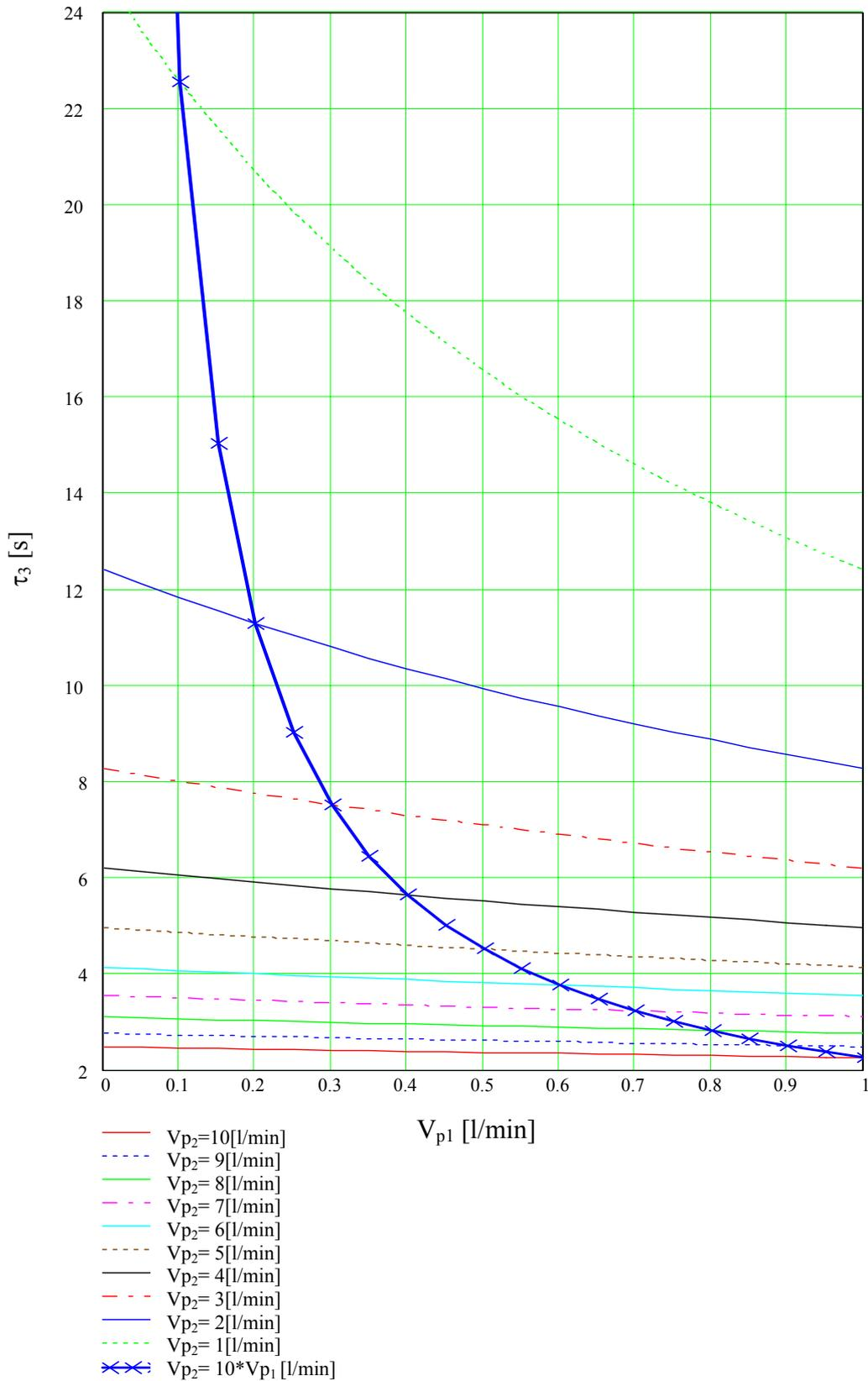
Figure 28 Residence time  $\tau_3$  for the SMPS DMA as a function of the sample flow  $V_{p1}$  and the sheath flow  $V_{p2}$ . As a recommendation from TSI the ratio of sheath flow to sample flow should be at least ten. The residence time for this ratio is shown with the thick blue line.
