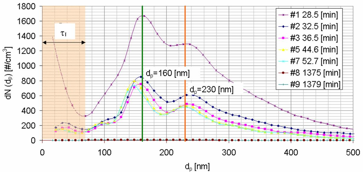
Figure 31 Monodisperse CMD measurement of the CAST setting  $d_{pg}=160$  [nm];  $\tau_1$  is the residence time before the aerosol flow enters the measurement site of the SMPS Classifier (experiment #65).
