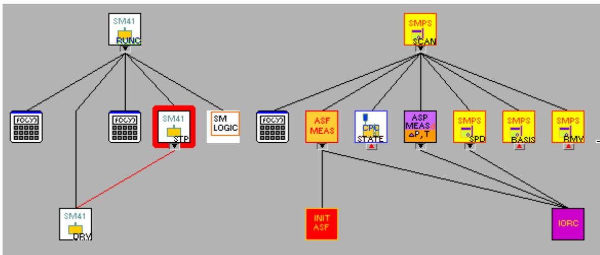
Figure 53 Program hierarchy for SMPS\_SCAN\_CPCXX.vi and SM\_RUNC.vi; Both programs are implicitly sub vi's of CMDC\_Measurement.vi and therefore not shown in Figure 51.
