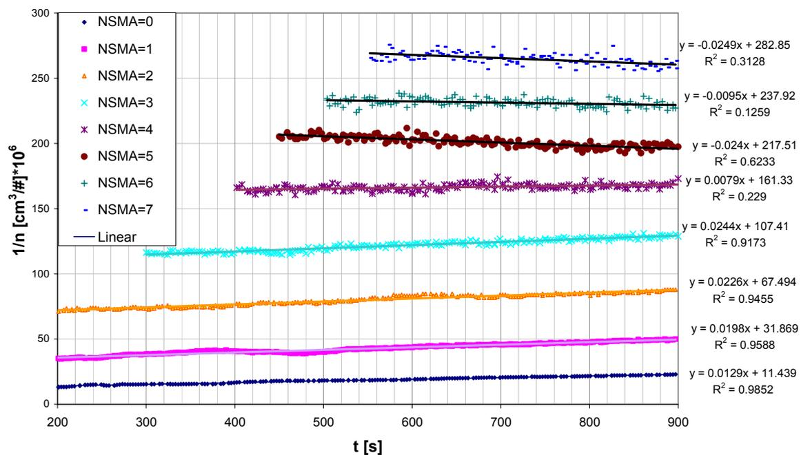
Figure 42 Smoluchowski plot of experiment #119; The particle source were – 4 candles with the flavor OP
