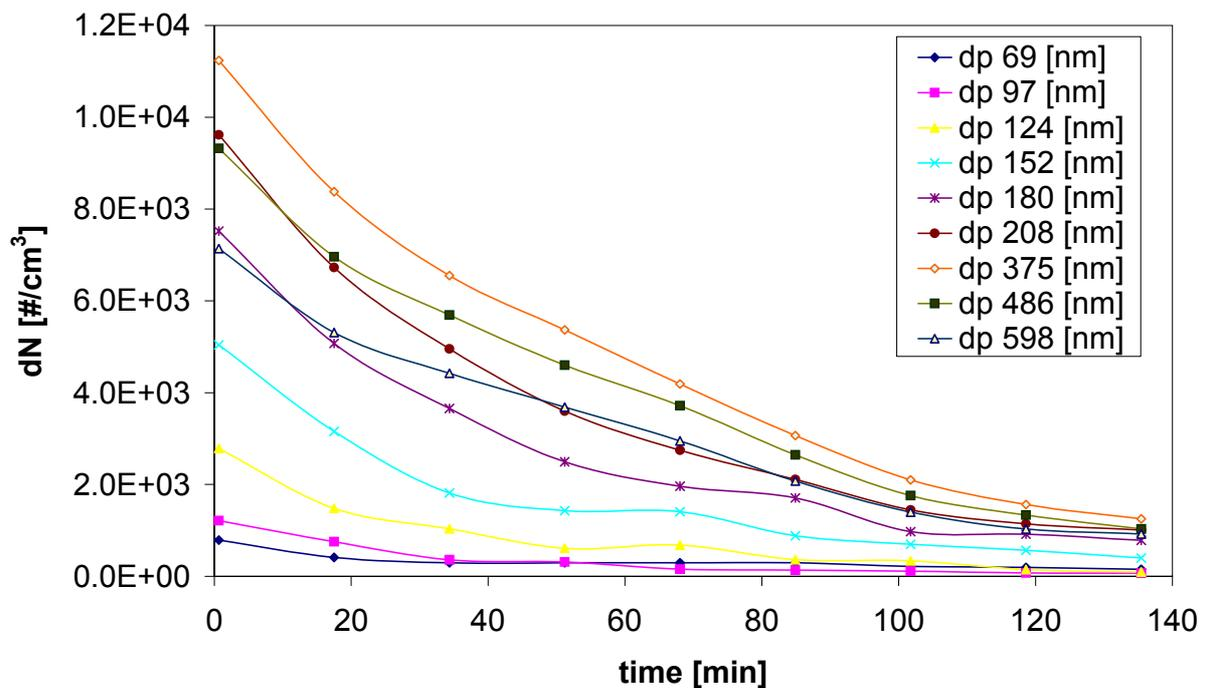
Figure 37 Evolution of the sized distribution of different particle sizes over time measured with the CMD for incense and nine sequential runs NSMA=1..9 in the CMD operation "Polydisperse Coagulation".  $dN$  is the particle size measured with the CPC plus the correction for the dilution and  $d_p$  is the mobility particle diameter in nm (This is a different view of Figure 38).
