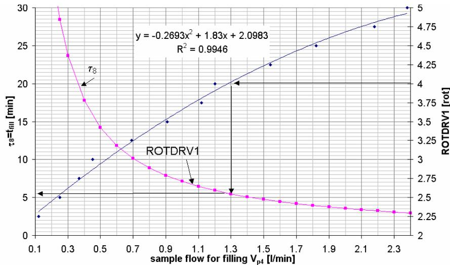
Figure 26 Minimum filling time for the settler  $\tau_8$ . The total settler volume was assumed with  $V_{70}=7.05$  [l], the volume for the settler and the gas path before was  $V_8=7.11$  [l]. On the right side the number of rotations, counted from the closed valve, of the needle valve DRV1 is related to the filling flow and hence to the minimum filling time  $\tau_8$  (see text for more details)
