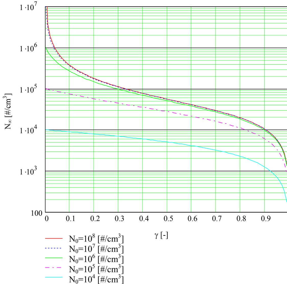
Figure 5 Solution of the logistic equation for the constant concentration reactor for different initial concentrations  $N_0$  and a constant emptying time  $t_{total} = 75$  [min] and the constants  $L_0 = 1.89 \cdot 10^{-4}$  [1/s] and  $= 56.7 \cdot 10^{-10}$  [cm<sup>3</sup>/s] according to equation (0-61)
