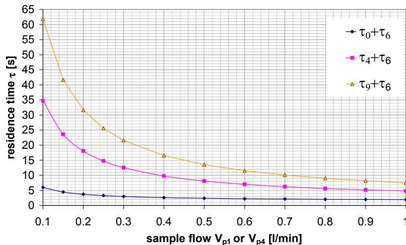
Figure 30 Residence times for the standard SMPS system  $\tau_0 + \tau_6$  and the CMD system  $\tau_4 + \tau_6$  or  $\tau_9 + \tau_6$  as a function of the sample flow  $V_{p1}$  or  $V_{p4}$
