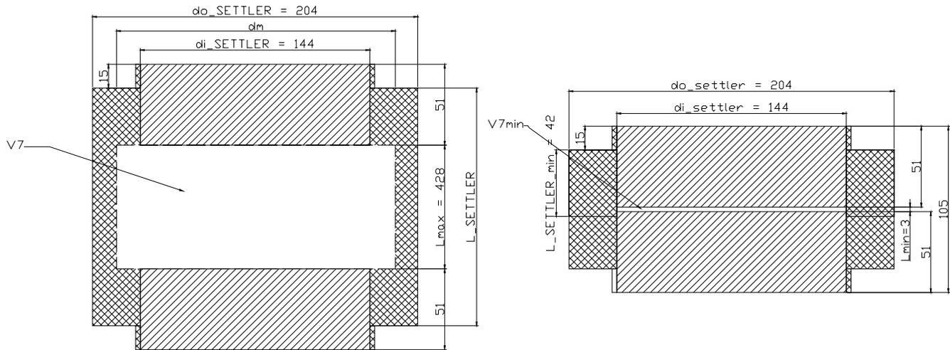
Figure 10 Settler in the end switch positions
