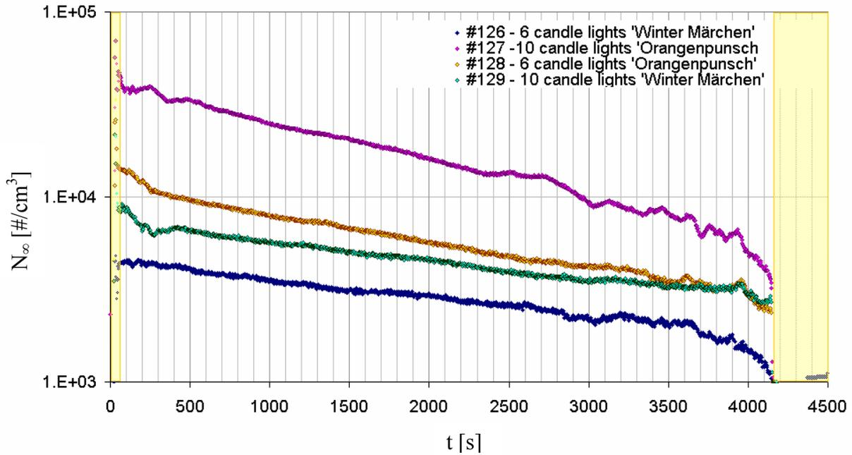
Figure 40 Raw data for experiments #126-#129: Test for operation “Polydisperse Coagulation I” for determination of the coagulation constant, for two different types of candle lights and two different concentrations; The candle light with the flavor “Orangenpunsch” produce higher particle concentrations  $N_\infty$  than the candle lights with the flavor “Winter Märchen”.
