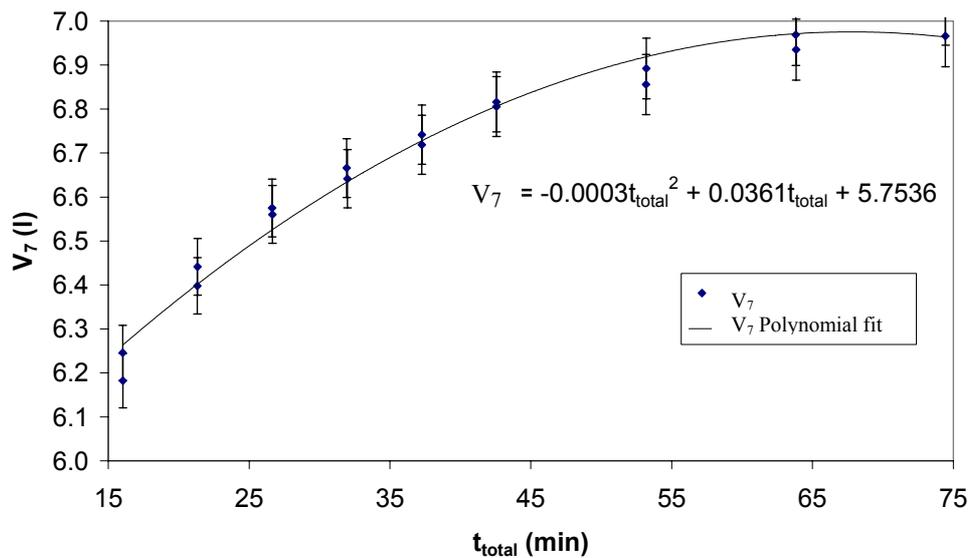
Figure 13 Calculation of the total effective settler volume according to the measurement in Figure 11 and equation (0-5).
