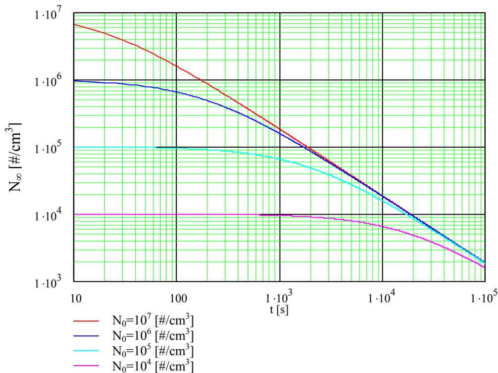
Figure 2 Solution of the Smoluchowski equation for different initial concentration and a constant coagulation coefficient  $K=54 \cdot 10 \text{ cm}^3/\text{s}$ .
