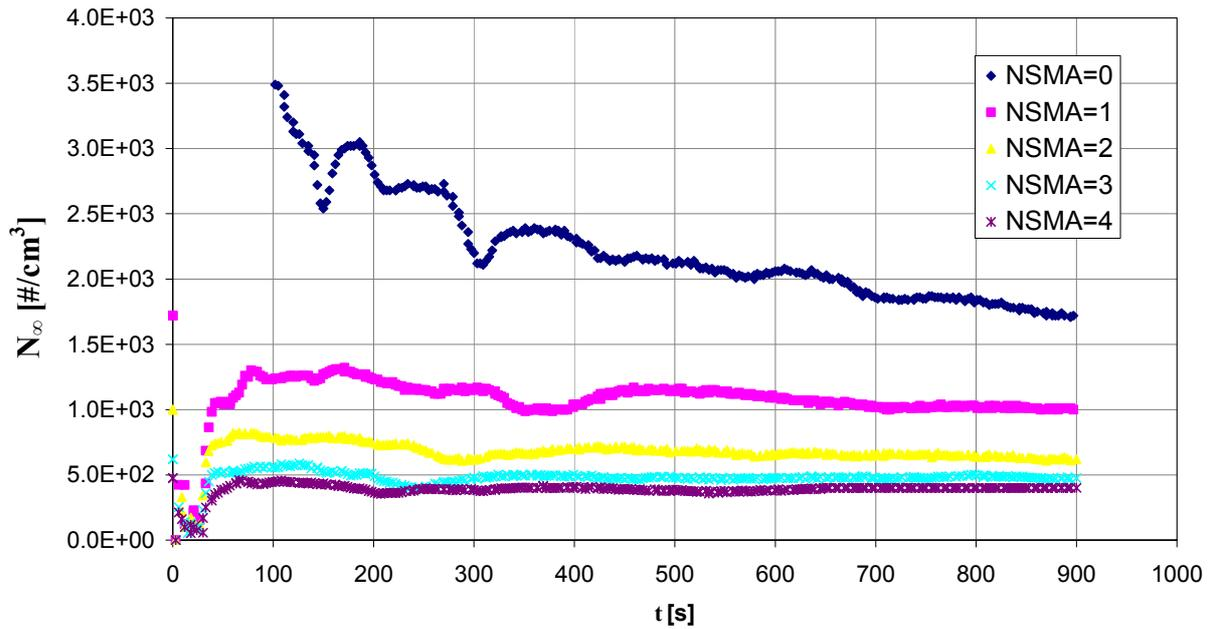
Figure 44 Number concentration  $N_\infty$  measured with the operation “Polydisperse Coagulation II” and experiment #121. The particle sources were 4 candles with the flavor WM; The residence time is not subtracted from the measurement time.
