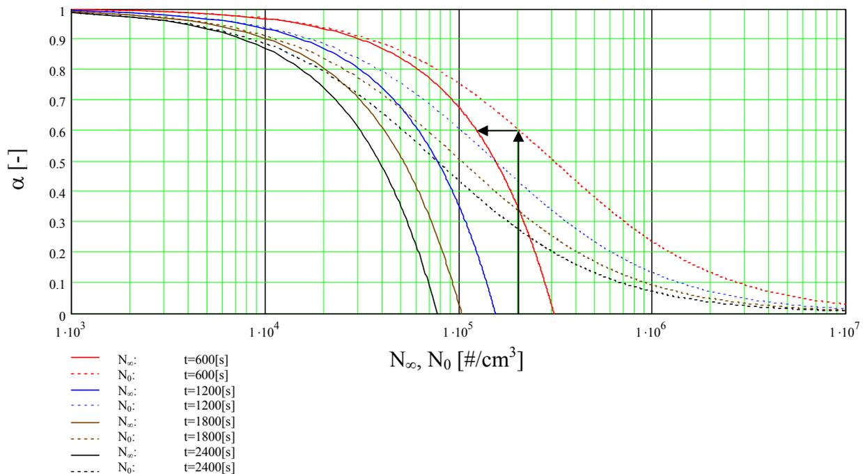
**Figure 3** Solution of the Smoluchowski equation for a different concentration decrease  $\alpha$  and the corresponding actual as the initial particle concentration  $N$  and  $N_0$ ; Different coagulation times  $t$  are used as a parameter. The coagulation coefficient is constant  $K = 54 \cdot 10^{-10}$  [cm<sup>3</sup>/s].
