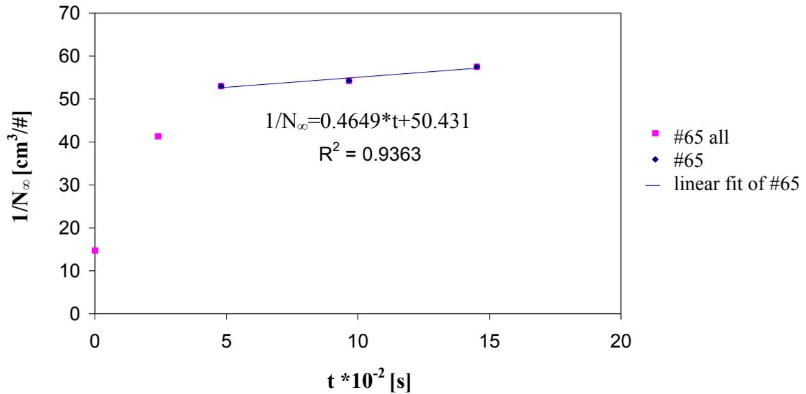
Figure 36 Smoluchowski coagulation plot for monodisperse soot measurements with the CAST;  $K_a = 4.649 \cdot 10^9$  [cm<sup>3</sup>/(#\*s)] (experiment #65).
