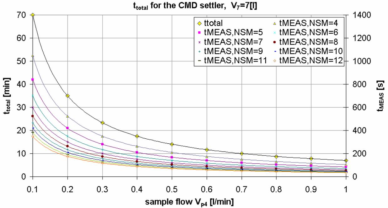
Figure 49 Total measurement time possible when emptying the settler as a function of the sample flow  $V_{p4}$  and the number of the measurements (NSM) on the right y-axis; The total measurement time as a function of  $V_{p4}$  can be read on the left y-axis (this Figure is similar to Figure 27 but also lower sample flow rates can be seen)
