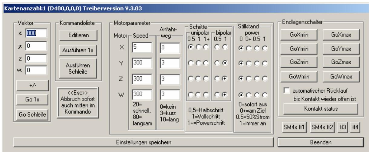
Figure 54 Standard application “SM4xDRV.EXE” from Hasotec for the stepper motor control. Has to be started and closed before running the LABVIEW program to load the driver for the Hasotec driver card into PC-memory.
