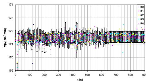
Figure 43 Volume flow  $V_{p4}$  for all measurements of experiment #121; The particle source were 4 candle lights with the flavor WM;
