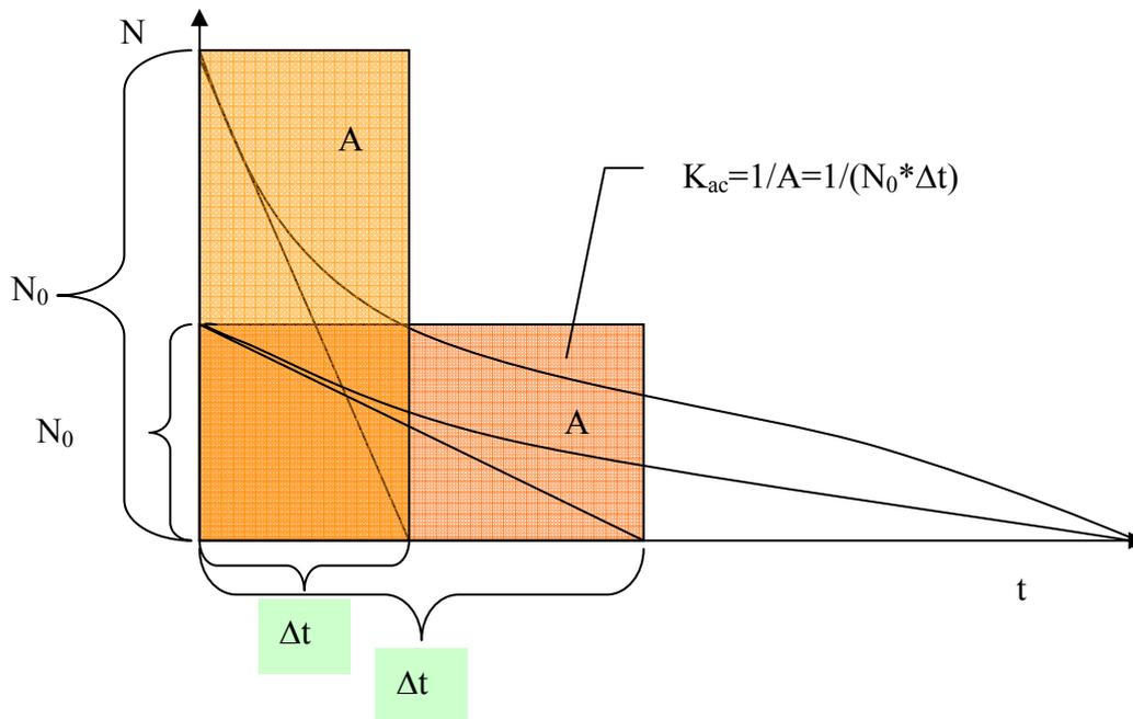
Figure 6 Graphical method to determine the apparent coagulation coefficient  $K_{ac}$  according to equation (0-67). The method is described in the text.
