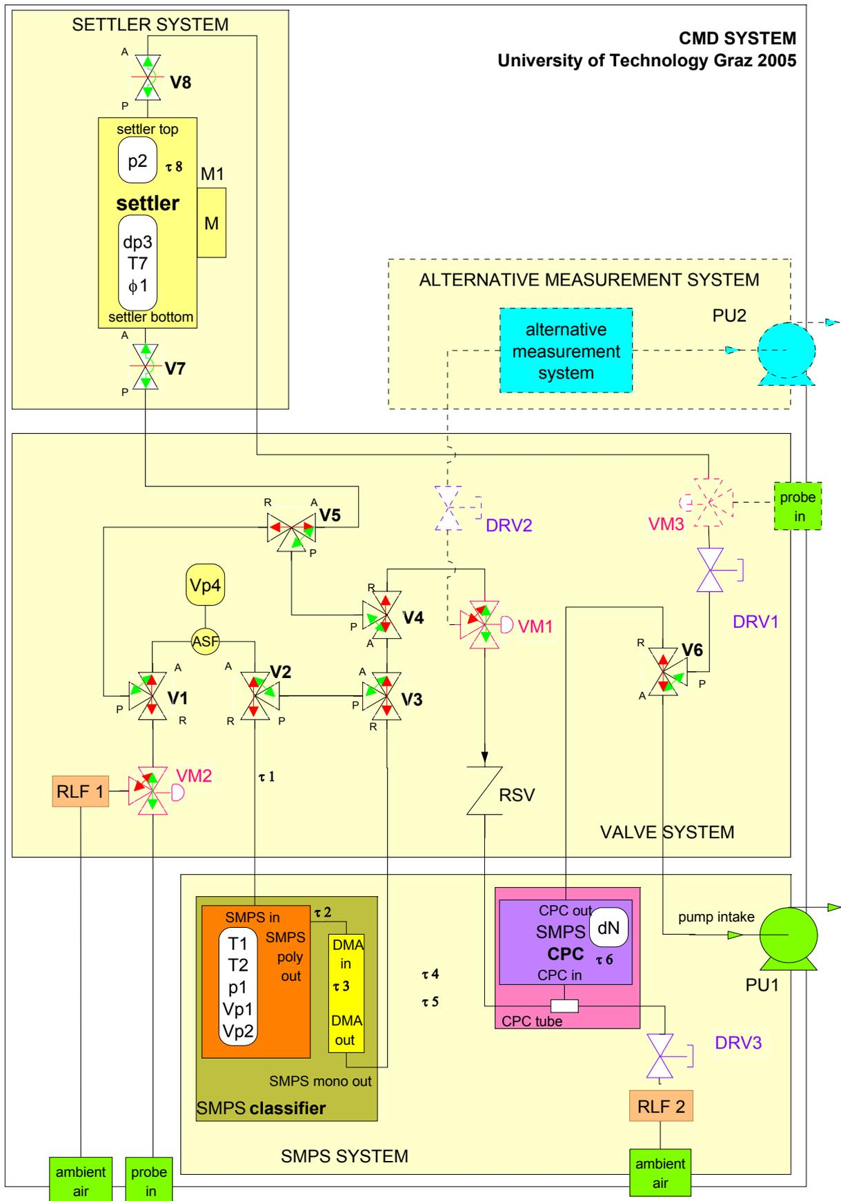
Figure 48 CMD flow chart with possible valve positions
