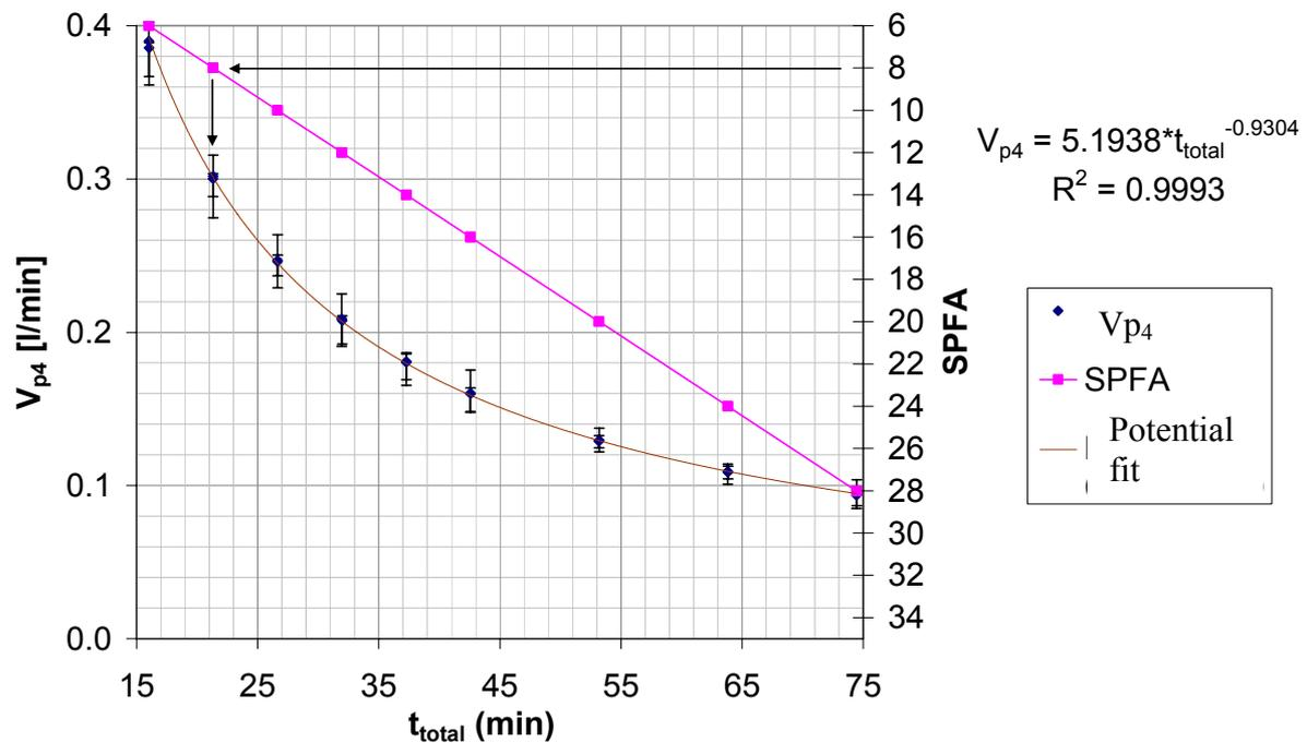
Figure 11 Flow rates  $V_{p4}$  of the flow sensor ASF 1430 for different times of emptying and filling the settler; The parameter SPFA denotes the speed factor of the stepper motor in the LABVIEW software. It is proportional to the stepper motor steps per time unit.
