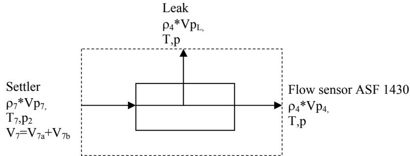
Figure 14 Scheme of the settler flow  $V_{p7}$  the leakage flow  $V_{pL}$  and the measured flow  $V_{p4}$  for the mass balance
