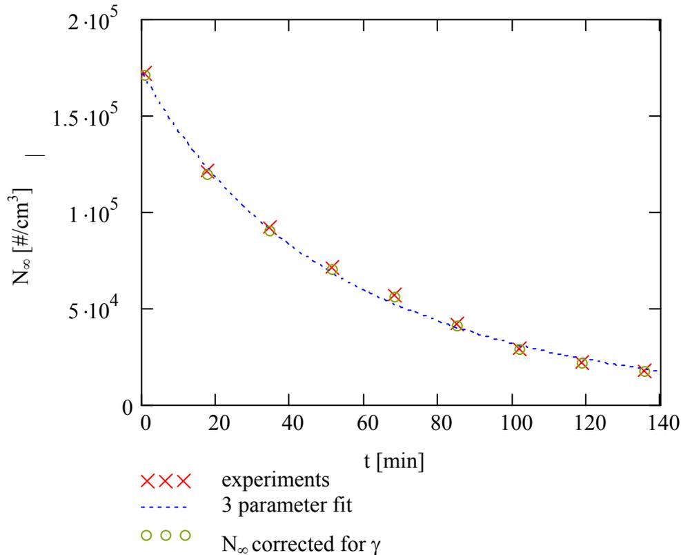
Figure 39 Particle concentration decay of the incense measurements. The experimental values (crosses) are corrected for the particle concentration according to the position of the settler (circles). A three parameter fit of equation (0-47) and  $N_\infty$ ,  $K$  and  $L$  is depicted with a dotted line.
