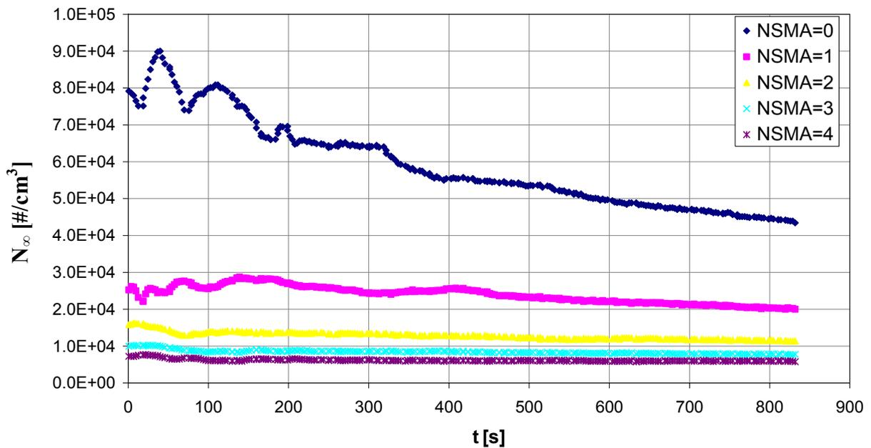
Figure 45 Number concentration  $N_\infty$  measured with the operation “Polydisperse Coagulation II” and experiment #119. The particle sources were 4 candles with the flavor OP; the residence time is already subtracted from the measurement time.
